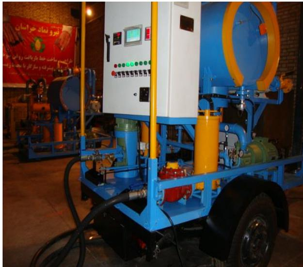
**Fig.1.** Representation of offline refinery device of hydraulic oil (filtration)
