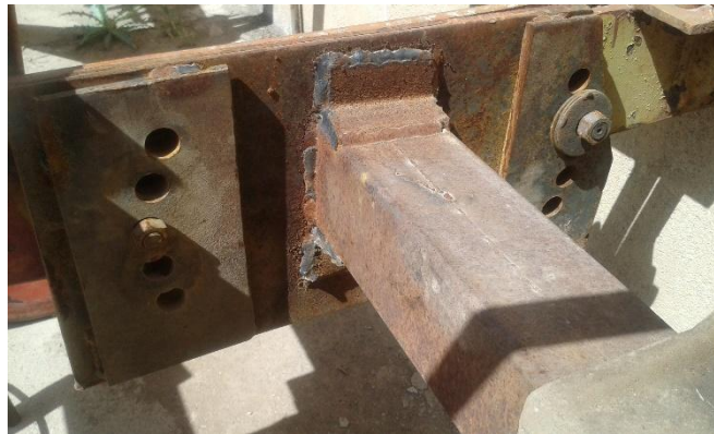
Fig.1. Mechanism for adjusting the rake angle
