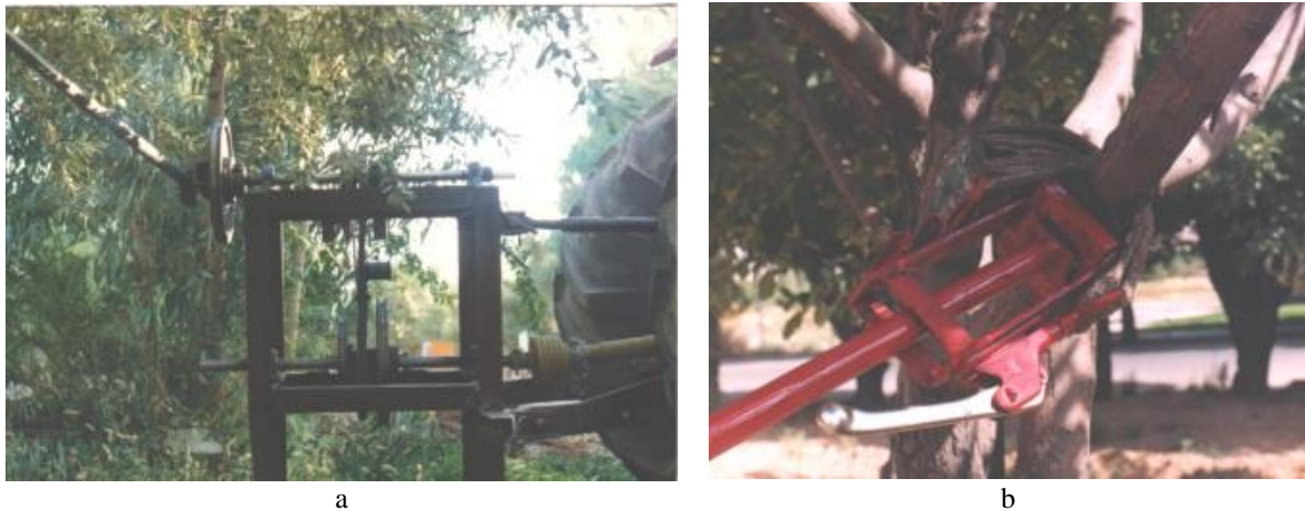
Fig.2. a) Fabricated limb shaker during evaluation in the orchard, b) clamping device with soft pad attached to limb for vibration cushioning.
