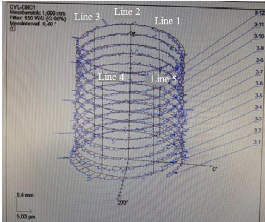
**Fig. 3.** The position of sections for roundness and straightness measurements
