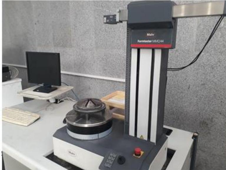
**Fig. 2.** The Formtester used for measuring dimensional and geometric specifications of cylinder liner. All dimensional and geometric specifications of the surface were evaluated with average values of five evaluation tests. The data were analyzed using descriptive statistics such as mean ( $M$ ), standard deviation ( $S_D$ ), and combined standard uncertainty ( $U_C$ ), which is calculated according to the Eq. (1).
