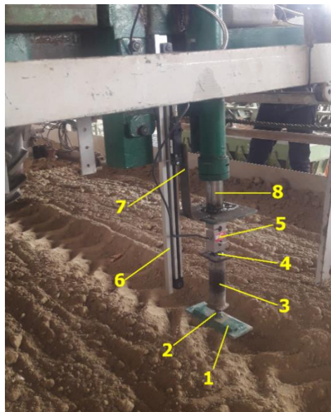
Fig. 5. A photograph of the bevameter mounted on the soil bin chassis: 1. Bekker Plate, 2. Screw, 3. Connection Rod 4. Screw, 5. Load cell, 6. MLC320 Linear Encoder, 7. Connector, and 8. Shaft
