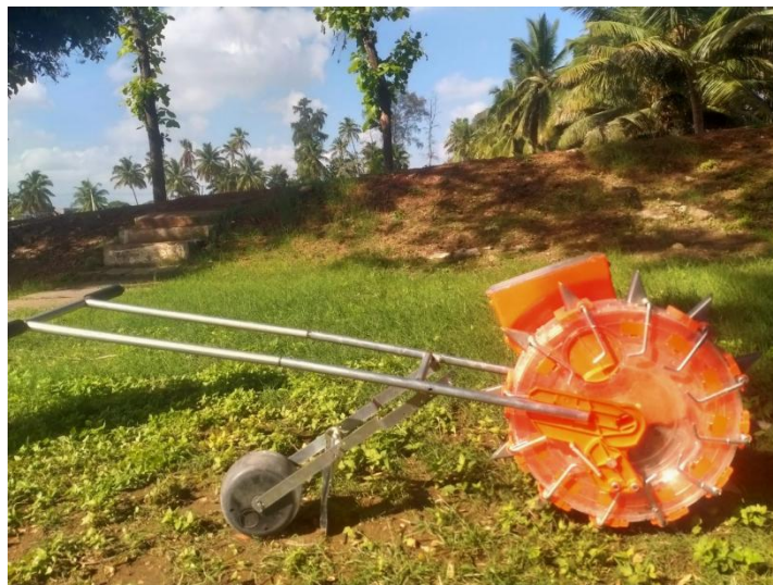
Fig. 1. Hand-held rotary dibbler
