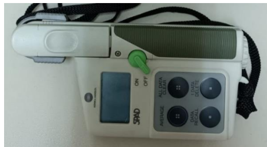
Fig. 3. SPAD measurement device
