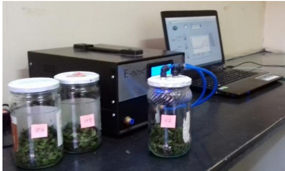
Fig. 1. (Left) The e-nose system, which comprises a sampling chamber, a system equipment box, and a computer, and (right) a schematic block diagram illustrating the components of the e-nose device
