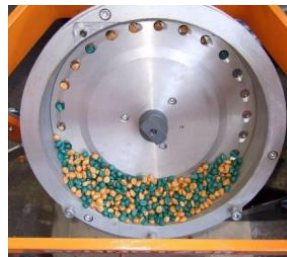
(g) Inclined Disk Seed Metering Device
