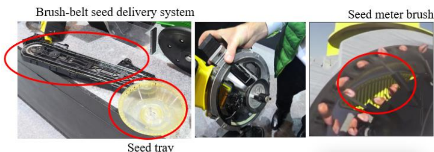
Fig. 8. John Deere pneumatic precision seeding system
