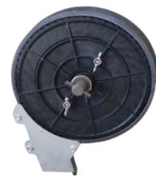
(h) Brush-Type Seed Metering Device
