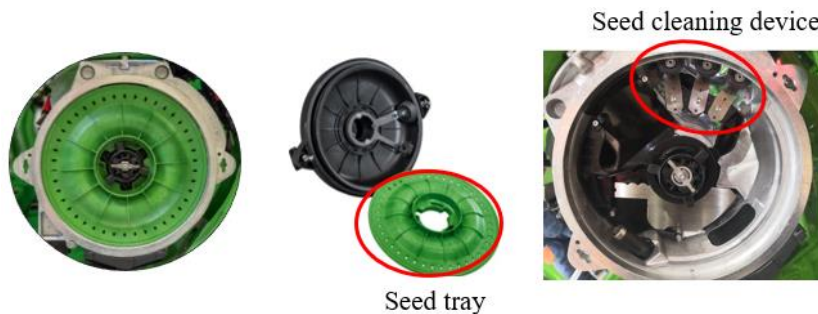
Fig. 6. Amazone positive-pressure seed metering apparatus
