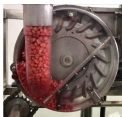
(a) Spoon-Wheel Seed Metering Device
