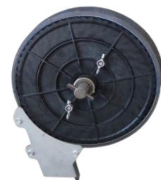
(h) Brush-Type Seed Metering Device
