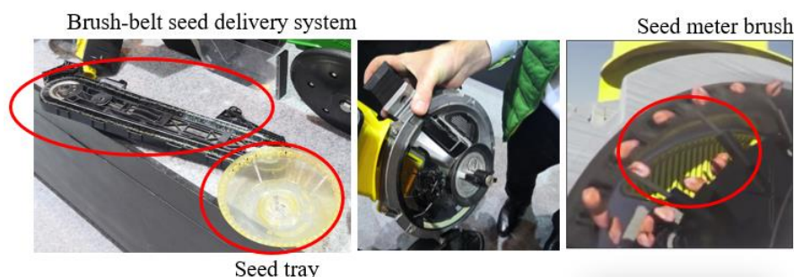
Fig. 8. John Deere pneumatic precision seeding system
