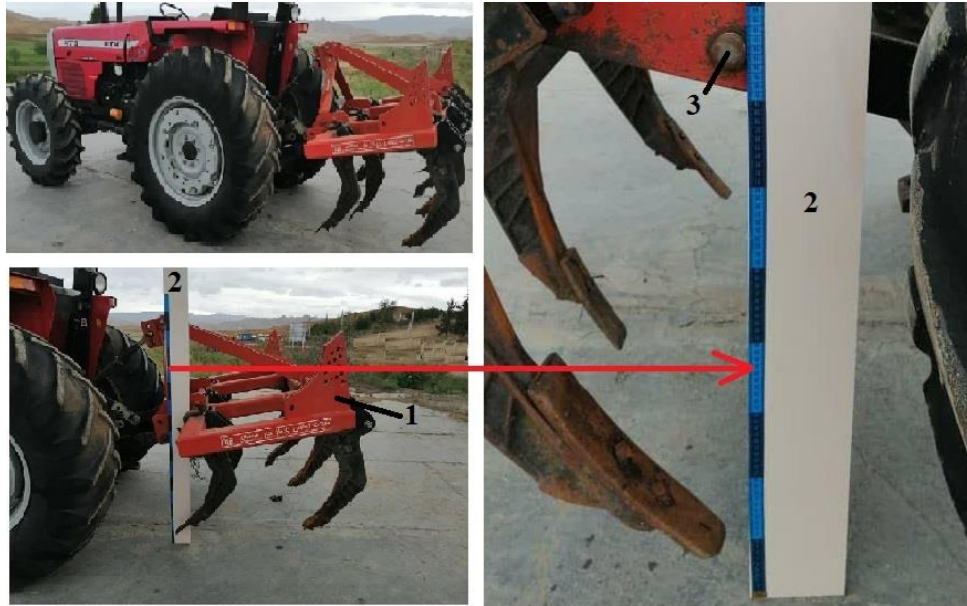
Fig. 2. Laboratory test setup on the Massey Ferguson tractor Model 475: 1= Chisel plough, 2= Set square ruler, 3= Connection pin between the lower arm and chisel plough.
