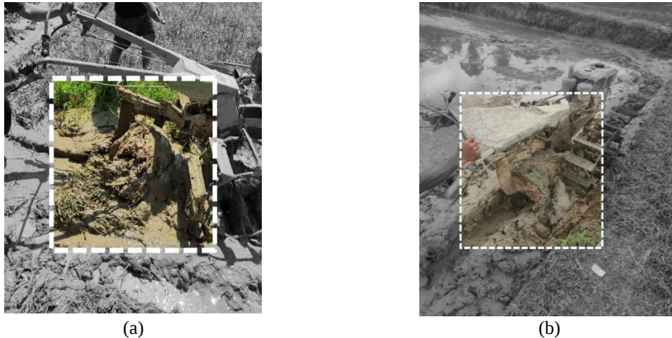
Fig. 5. Wheel Slip at (a) Low and (b) High speeds
