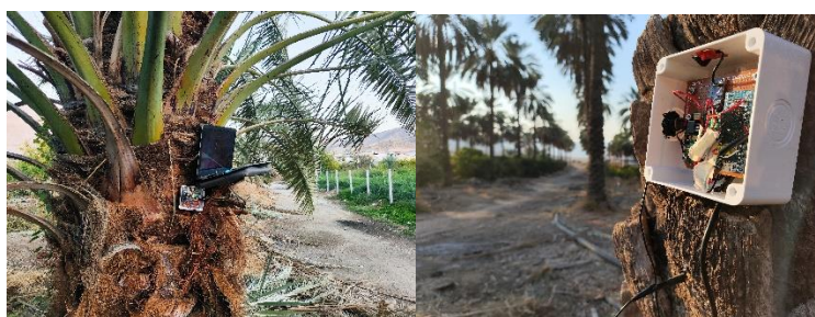
Fig. 2. Field-deployed acoustic sensing system showing the protective housing and microphone setup on an infested date palm trunk.
