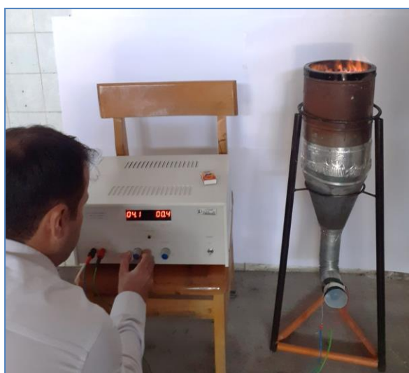
Fig. 4. Rice husk gas stove and flame adjustment using air velocities of 0.6, 0.7, and 0.8 \text{m s}^{-1}
