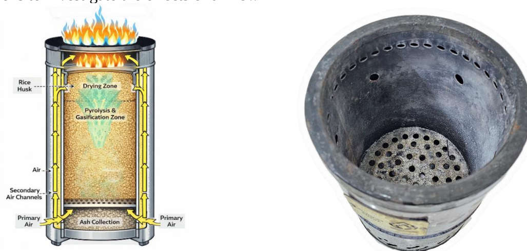
Fig. 1. Schematic view (left) and interior view (right) of the Bioheat brand biomass stove used in this study
