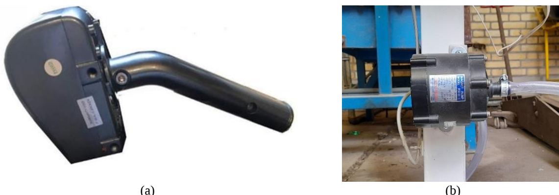
Fig. 4. (a) Electric motor of the sun tracker, and (b) the water pump used
