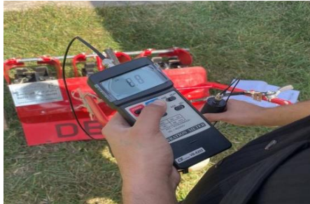
Fig. 3. The VB-8202 vibration meter and its technical specifications
