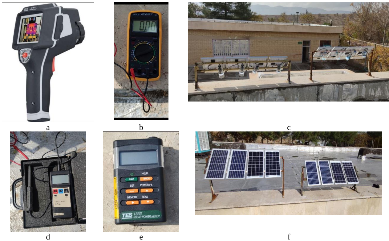
Fig. 1. a) CEM DT-9875 thermal camera, b) Digital multi-meter, c) Back view of PV modules, d) Hygrometer, e) Pyranometer, and f) Front view of PV modules
