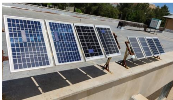
Fig. 3. Creating artificial shadow on the hot cells of the panels
