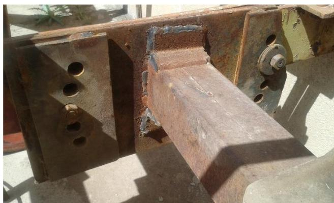
**Fig.1.** Mechanism for adjusting the rake angle
