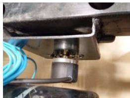
Fig.5. Rotary encoder mounted on rotating shaft
