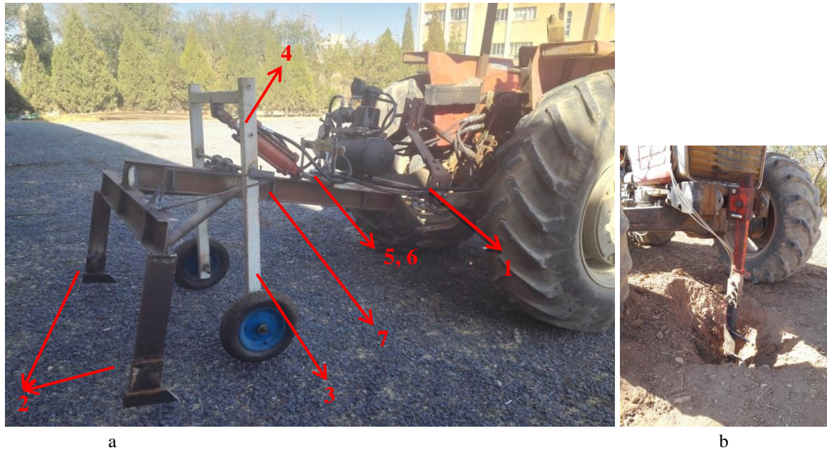
Fig. 2. a) View of VDT tool; 1) main chassis and three-point hitch, 2) tine, 3) wheels and wheel axles, 4) double-sided cylinder, 5) 4/3 Directional control valve; 6) Electric motor pushing hydraulic valve lever, and 7) Shaft encoder; b) the pneumatic sensor
