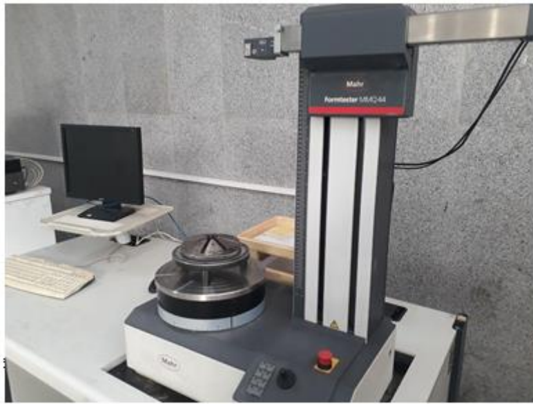
Fig. 2. The Formtester used for measuring dimensional and geometric specifications of cylinder liner
