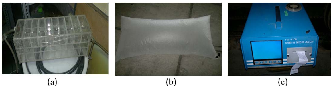
Fig.2. (a) Gas mixing chamber, (b) Voluminous air bag (bates cargo pack), (c) Automotive emission analyzer
