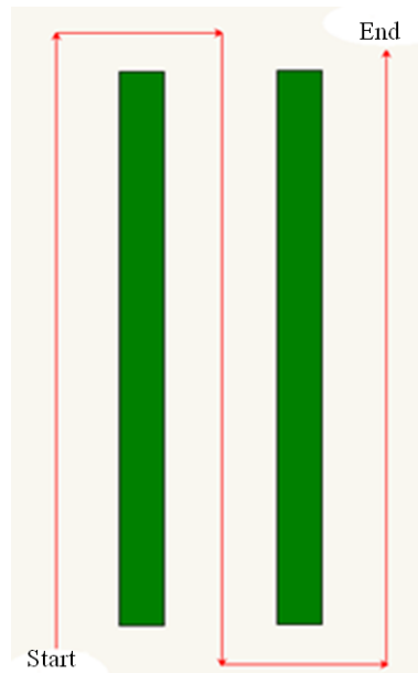
Fig.3. Rows of plants in a greenhouse and robot moving route
