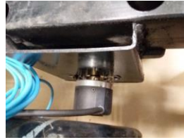
Fig.5. Rotary encoder mounted on rotating shaft
