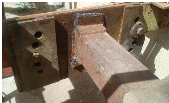
Fig.1. Mechanism for adjusting the rake angle
