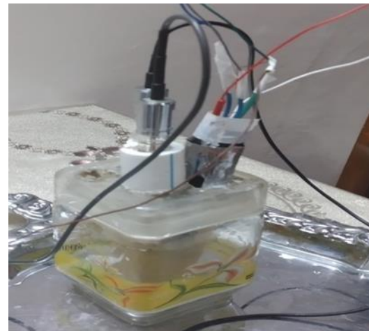
Fig.5. Electrodes including gold, platinum, palladium, titanium, and silver as working electrode, Ag/AgCl electrode as reference, and platinum electrode as counter electrode
