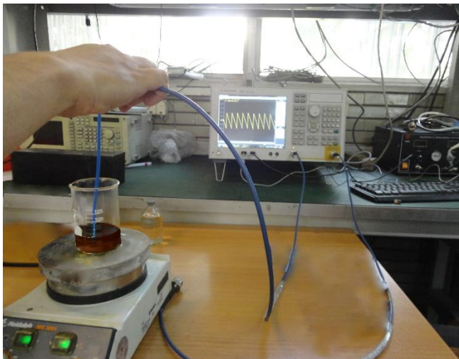
Fig. 3. Experimental and schematic setup for dielectric properties measurement
