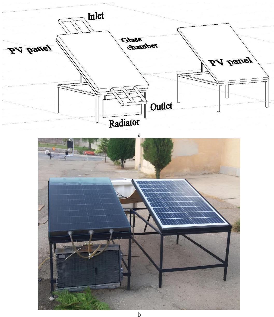
Fig. 1. The reference panel and PVT system developed in this study: (a) schematic diagram, and (b) the real image
